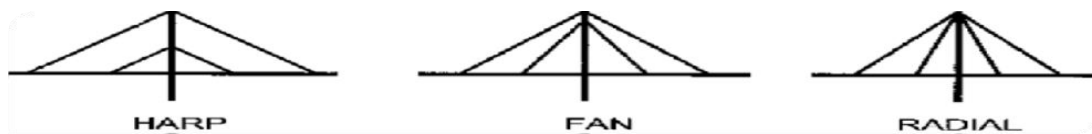
(Fig no.9 Major Classes of Cable-Stayed Bridges)
